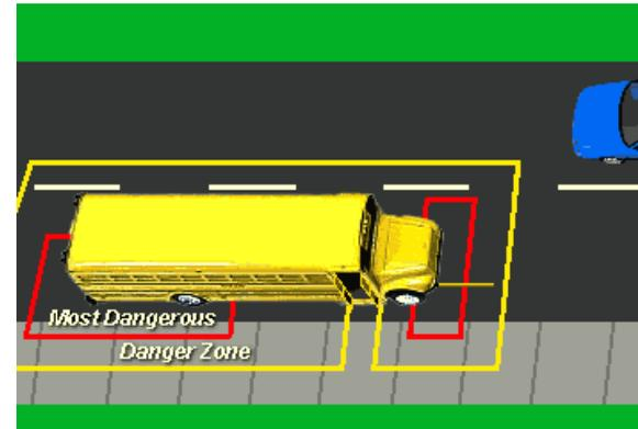
The danger zone exists as a 10 feet all around the bus—the most dangerous areas include the front of the bus and the right rear tire area.
